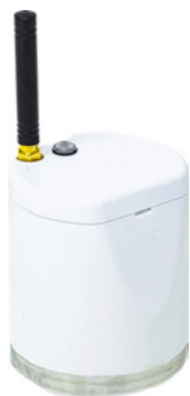
Figure 6. Wireless vibration monitoring evaluation platform.
