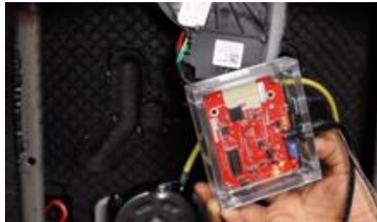
Sensor inside the seat
