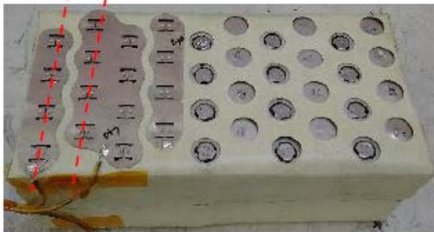
圖 10a. TRP occurred slowly due to air flow thermal conductivity and low ability store heat
