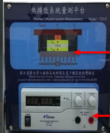
Power supply of thermal diffusivity measuring instrument
