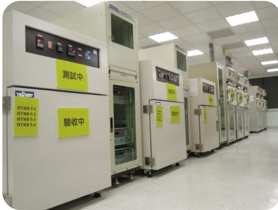
HTRB ( High Temperature Reverse Bias Taster )
