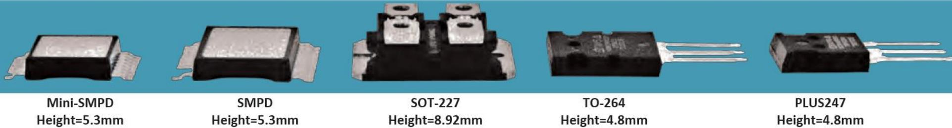
The above accentuates the compact and low profile nature of the device. Compared to a conventional high power package such as the SOT-227, the IXYS SMPD features  $\frac{1}{4}$  the weight and  $\frac{1}{3}$  the volume and provides similar electrical and thermal characteristics.
