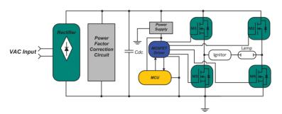
High Intensity Discharge (HID) lamp ballast
