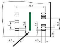
A slit in the board may be used for board stress relief
