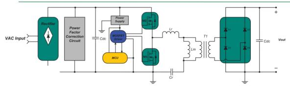
**SMPS - Half-Bridge Resonant-Mode Converter**
