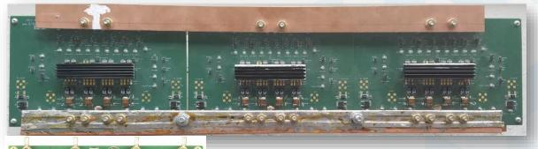
FPGA Core 0.8V @100A Power Supplier Solution
