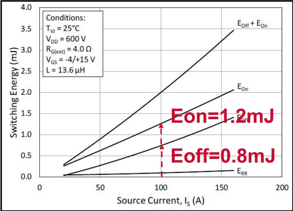
Figure 11. Switching Energy vs. Drain Current ( $V_{DS} = 600V$ )
